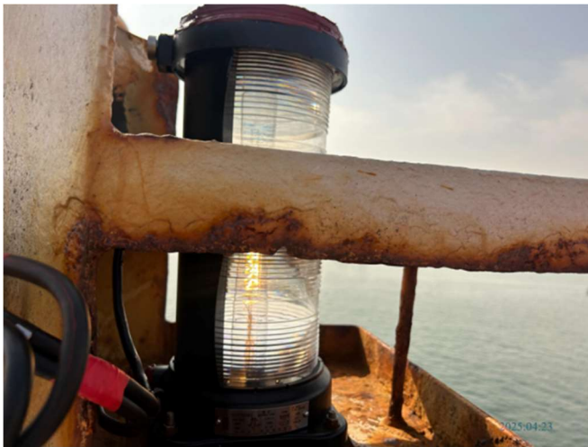
The horizontal light arc of mast light on top of the forecastle not complying with requirements of COLREG.
